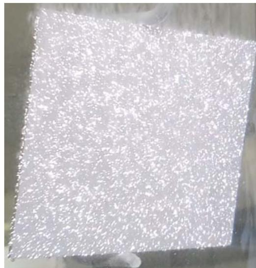
**Fig. 2: Characteristic plasma discharge on an aluminum sample**
