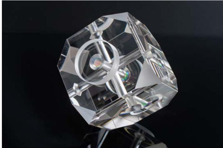
**Fig. 3: Ultra high-finesse optical cavity with a 50x50x50 mm<sup>3</sup> cubic spacer, crossed-axis boreholes, and magnetron sputtered mirrors contacted through optical contacting followed by USP laser micro welding.**
