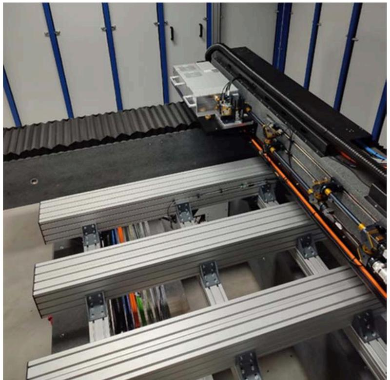
**Figure 2: Machine module RDX2800 with ultrafast laser for parallel processing of a workpiece with dimensions 2.5m x 1.5m.**
