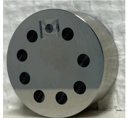
Figure 6: A 5x5 mm fused silica sample welded to Kovar
