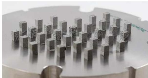
**Figure 1. 3 mm x 3 mm x 3 mm pure Molybdenum cubes still attached on the built platform via a 2.5 mm high support structure.**
