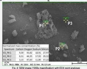
Fig. 4: SEM image (1959x magnification) with EDX point analyses
