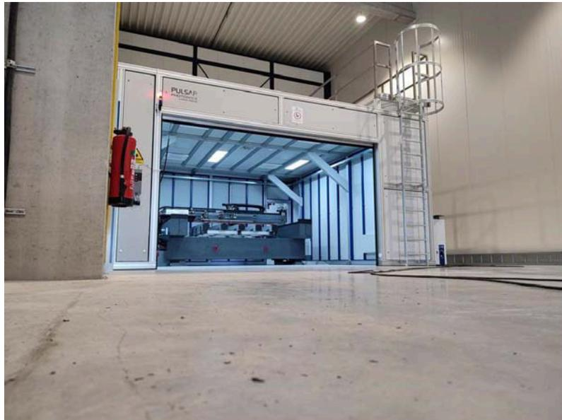
**Figure 1: Modular gantry system RDX2800 for large area laser processing with ultrafast lasers.**
