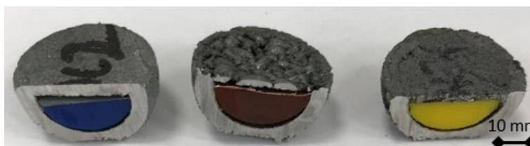
**Figure 6: Cut samples with glued sensor dummies; left - with aluminium adhesive tape; centre - with copper adhesive tape; right - with aluminium-bitumen-tar adhesive tape**
