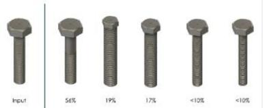
Figure: Input of hex screw STL model from the FabWave dataset and similarity scores of best matches
