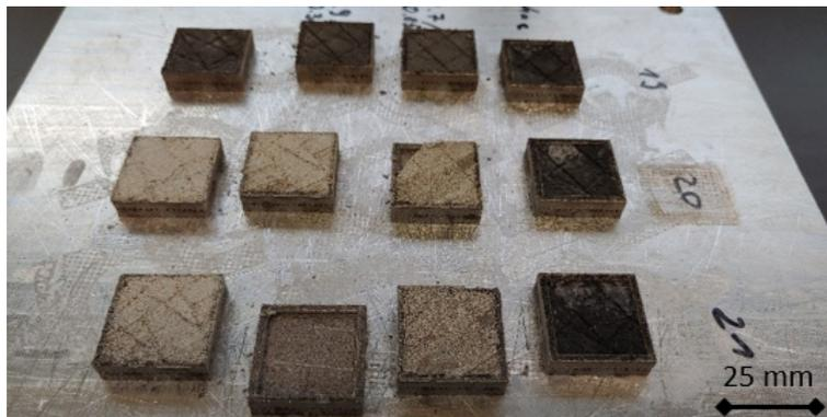
**Figure 5: Cast cavities after exposure; grey surface - powder cavities; dark surface - cavities with epoxy resin**
