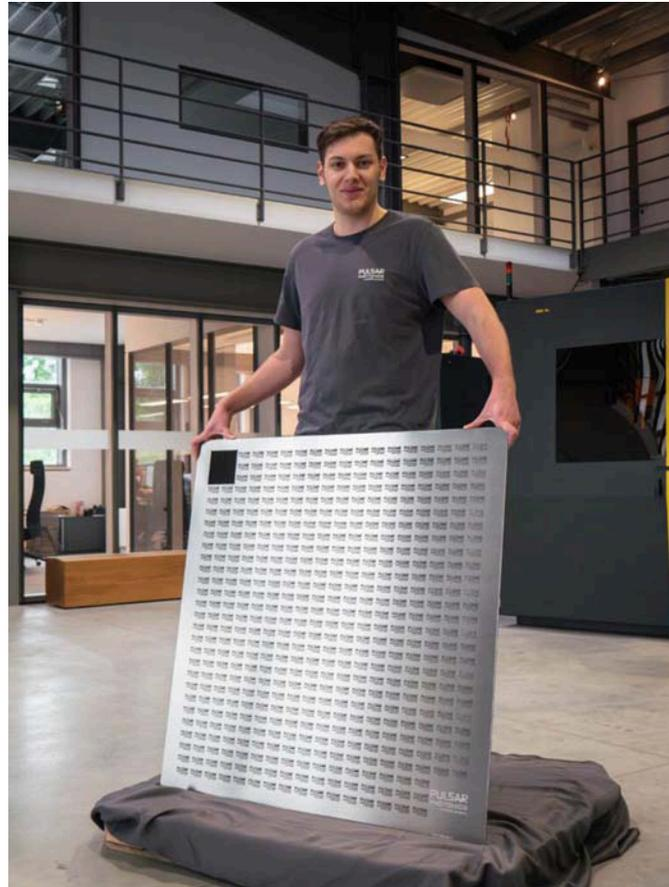
**Figure 3: Demonstrator plate (1000 mm x 1000 mm) for large-area USP laser processing with sample structures for functional surfaces and deep engravings.**
