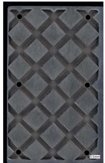
**Figure 4: Combined processing using ultra-short pulse (trenching) and water-jet guided technology (drilling) from SiC.**
