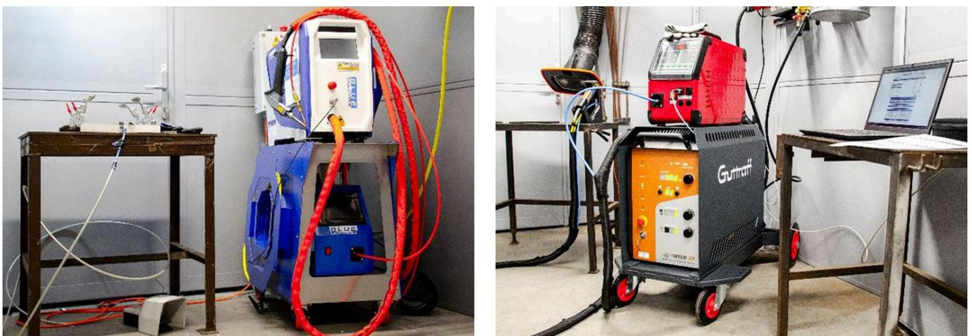
Figure 1: Two different handheld laser welding systems
