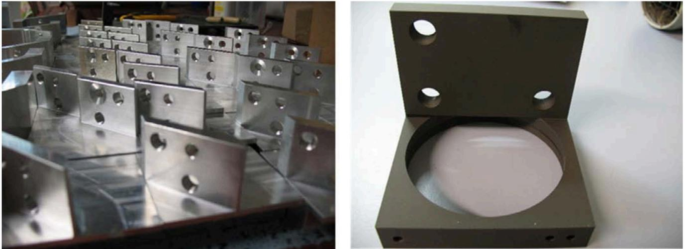
Fig. 4: Lens holder (left uncoated, right PCO coated)
