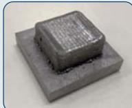
The multi-layer metal deposition process of a cuboid with an edge length of 30 mm was monitored. 14 infill tracks are combined with 2 border tracks. A uni-directional scanning strategy was used. The entire welding path was rotated 90° layer by layer.
