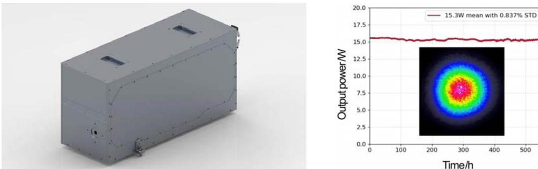
**Abb. 1: Left: Rendered view of the activeTwo-15. Right: Long term measurement of output power. Inset shows beam profile at full output power**
